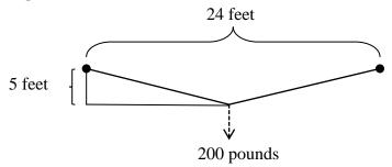
Solution: (e) We note that the triangle formed by the force F acting along the cable with the horizontal and vertical forces is proportional to the 5:12:13 right triangle whose hypotenuse is formed by the cable. Each anchor supports exactly half of the 200 pound weight by its vertical component. Therefore, the induced force F along the cable satisfies the proportion
