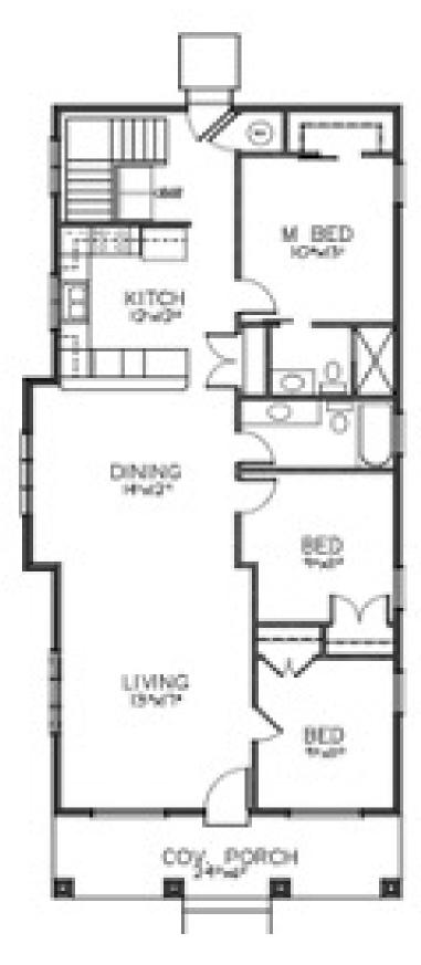
The home is long and narrow, therefore long site lines were designed to allow the feeling of a more open floor plan. All upstairs hallways were eliminated to open up the spacious feel of the floor plan and to accommodate for ADA accessibility.
