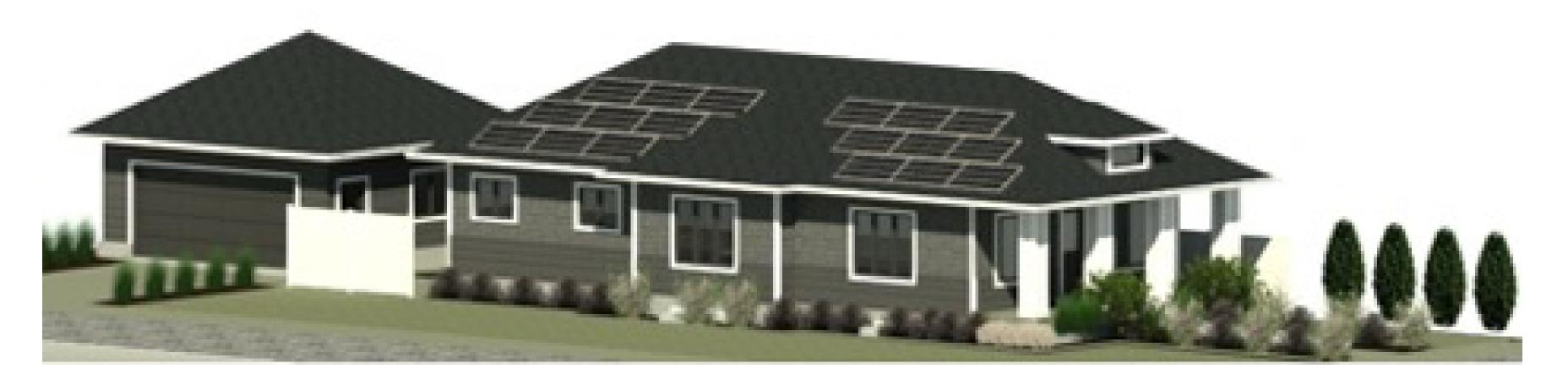
We designed large overhangs to nearly eliminate solar heat gain in the summer due to shade angles. We maximized the windows on the East side to allow solar heat gain in the winter, but limited the west facing windows and eliminated all windows on the south to minimize solar heat gain during the summer.
