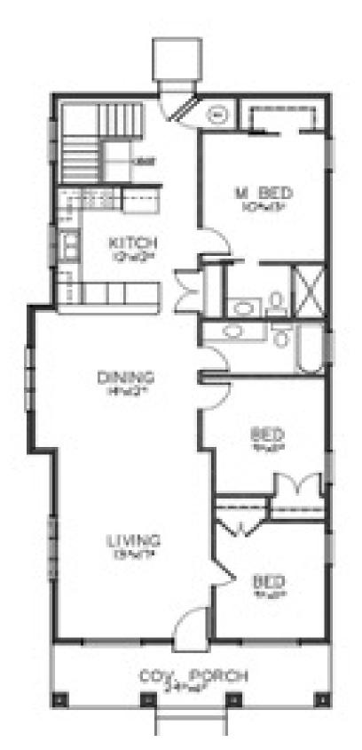
The home is long and narrow, therefore long site lines were designed to allow the feeling of a more open floor plan. All upstairs hallways were eliminated to open up the spacious feel of the floor plan and to accommodate for ADA accessibility.
