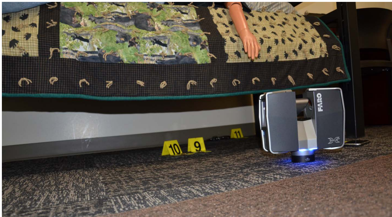
Figure 14: Photo taken by Darwin Little at the WSU practical, showing the FARO scanner head removed from the tripod and placed on the floor, ready to scan items at a lower point of view, such as under the bed. One possible problem is that the carpet may allow the scanner head to vibrate. Additionally, shadows and exposure to light are different from one scan to another on different elevations when stitched together.
