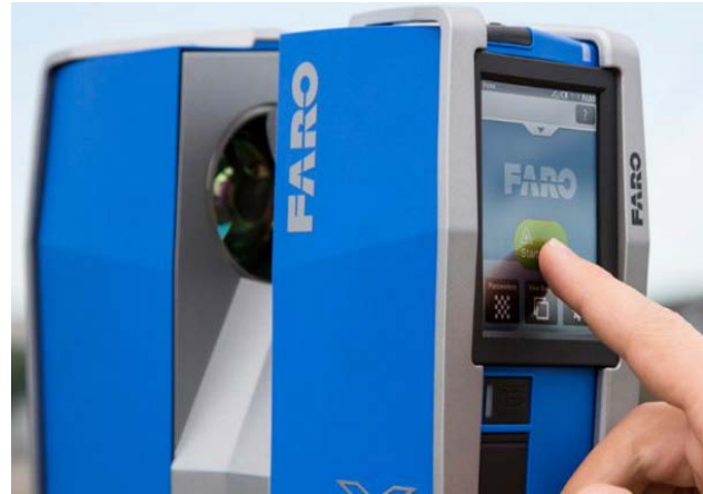
Figure 6: Readout controls located on one side of the FARO Focus scanner head. Retrieved 2018 from http://matrixti.com/matrix-on-manufacturing/3d-laser-scanning-industrial-plant-design/
