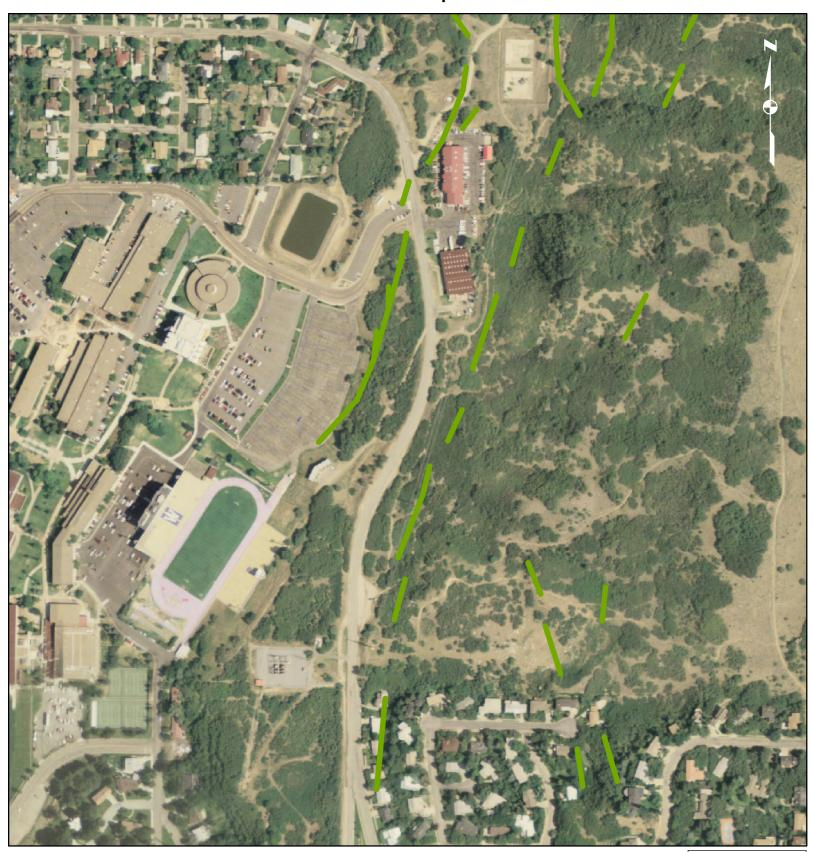
This map is to show how close the faults are to the construction site. As you will notice there are numerous faults that are running very close to WSU's campus. This close proximity to the faults makes the added cost of construction necessary.
