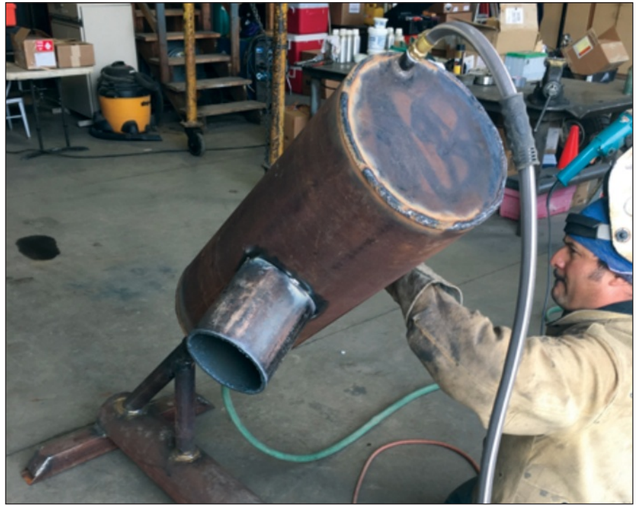
Fig. 3 — Welder testing for in-service welding.
