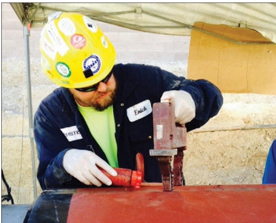
Fig. 4 — Magnetic particle testing (MT) of completed fillet welds on hot tap split sleeve.
