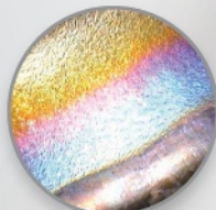
Heat Affected Zone and orbital weld inside a SS tube, viewed with a Hawkeye.
