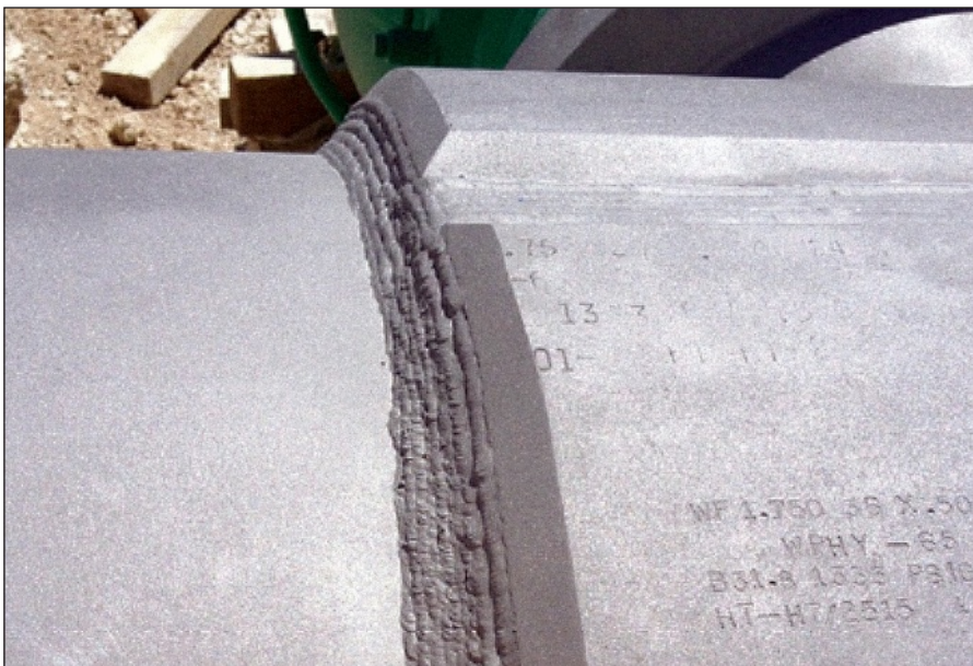
Fig. 2 — Billet markings on tap segments showing material specifications.
