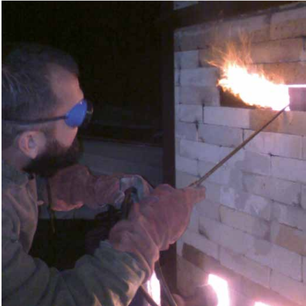
Spraying soda ash, soda kiln 2009
