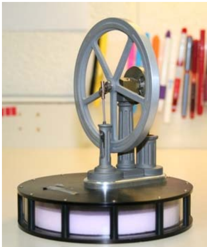
A senior project that was printed on the 3D Printer, and cast into metal at the local machine shop
