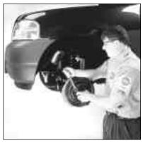
Step 1: Technician mounts an adapter to the hub.
