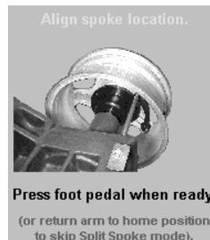
Rotate the wheel to position the Dataset<sup>®</sup> arm behind an adjacent spoke (nearest spoke in either direction). Enter the data by pressing the foot pedal.
