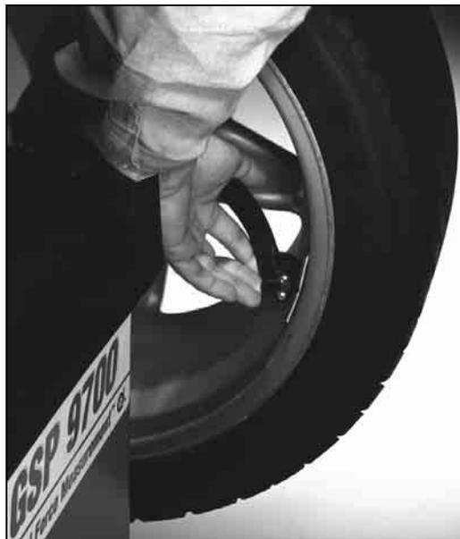
**NOTE:** If the servo is off (but is enabled in setup), pressing the “START” button with the hood in the RAISED position will restart the servo for adhesive weight application.
