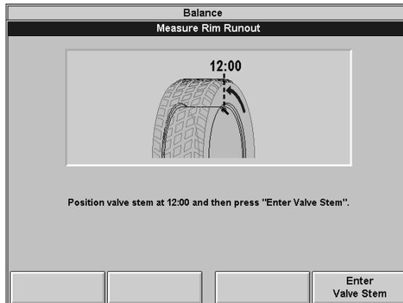
After measuring rim runout, you will be prompted to loosen the wheel and reclamp at one half turn (approximately 180 degrees) from the current position.
