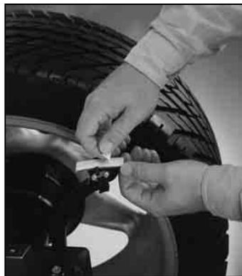
Using dimensional information previously obtained, the on-screen graphic displays and identifies the exact location of the weight plane and the current position of the inner Dataset<sup>®</sup> arm. Pull the inner Dataset<sup>®</sup> arm out from the base until the arm and the weight location are overlapping.
